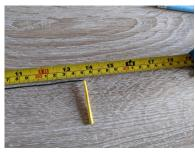
10. The point dibber can be used to measure the height of plant life in10cm intervals (using the marked points as a guide) along the horizontal frame. Smaller intervals can be surveyed by adding additional markers onto the
