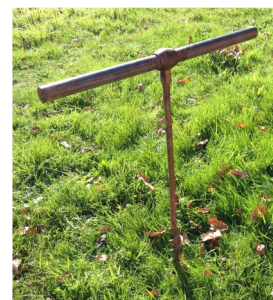
A soil auger partially screwed into the ground
