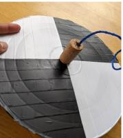
7. The underside of the disk needs to be weighted when in use to ensure the disk does not float on the surface of the water. In this example, a fabric bag weighted with a stone is attached to the screw eye using a carabiner clip, but any form of convenient weight can be used.
