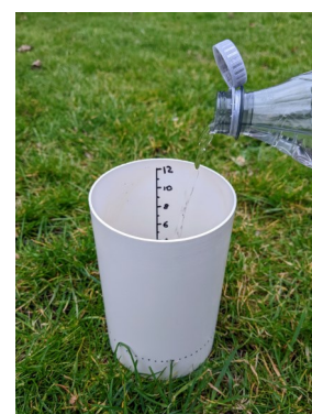
A homemade infiltrimeter
