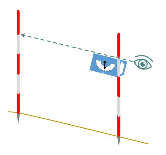
The gradient for that section of the ground, between the two ranging poles can then be read off the clinometer, and the process repeated along the length of entire transect. Gradients that are going up-slope are recorded as positive integers, while gradients going down-slope are recorded as negatives. Where students measuring every change in the angle of slope (example number 2 above), they should also measure the distance between ranging pole and record this alongside the gradient.
