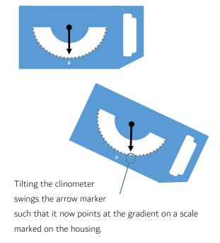
The user then places the top of the clinometer at the separation point between the red and white markings on the first ranging pole. It should be angled such that the clinometer is pointing directly at the same point on the opposing ranging pole and users should look directly along the top of the clinometer to ensure this is the case.
