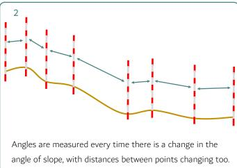
Regardless of how the transect is sectioned out, the method of measuring the angle of slope between each point is the same. One requires two ranging poles and a gun clinometer as well as a tape measure. The tape measure is laid out such that it stretches from one end of the transect to the other.
