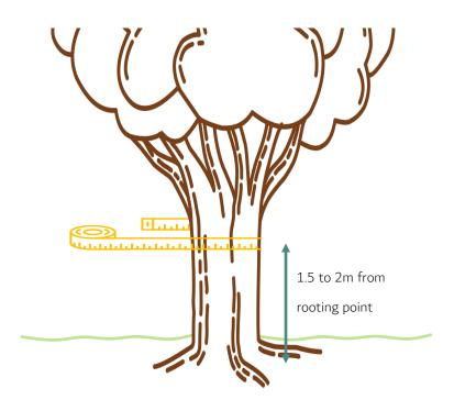
The tape measure should be pass freely around the trunk with no obstruction from branches, stems or knots.
